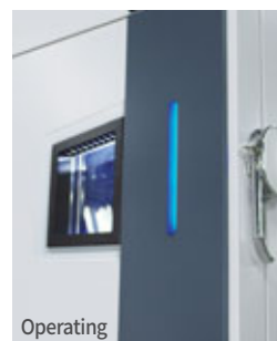
Indicator LED of operation condition
