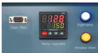
Electronic over temperature shutdown system.
