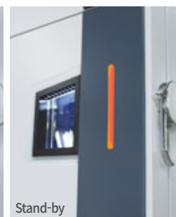
Indicator LED of operation condition
