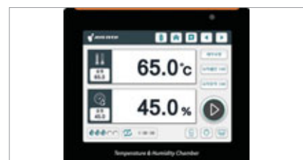
Controller for temperature and humidity control. (TH3-model)
